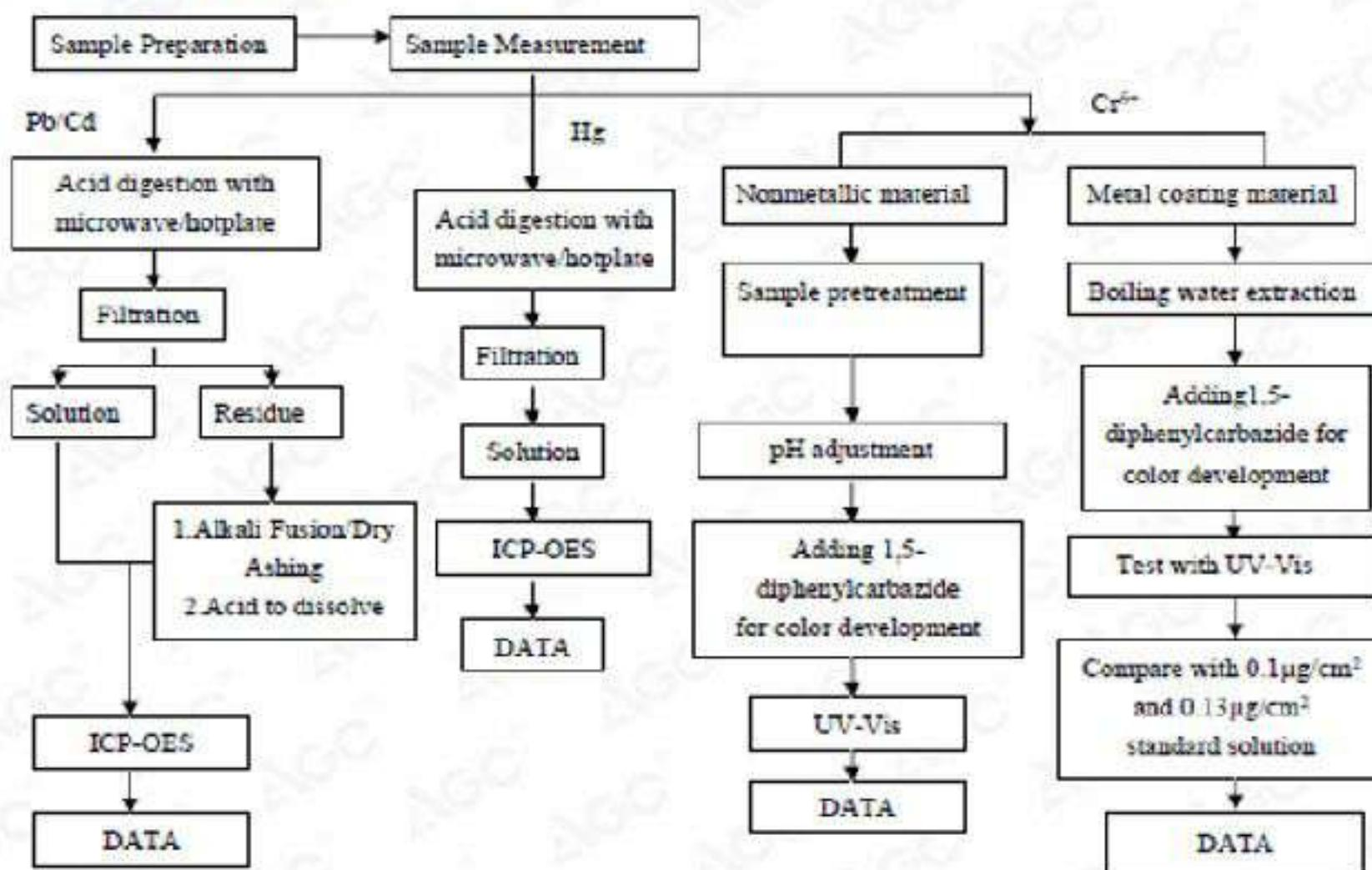
These samples were dissolved totally by pre-conditioning method according to above flow chart (Cr<sup>6+</sup> test method excluded)
