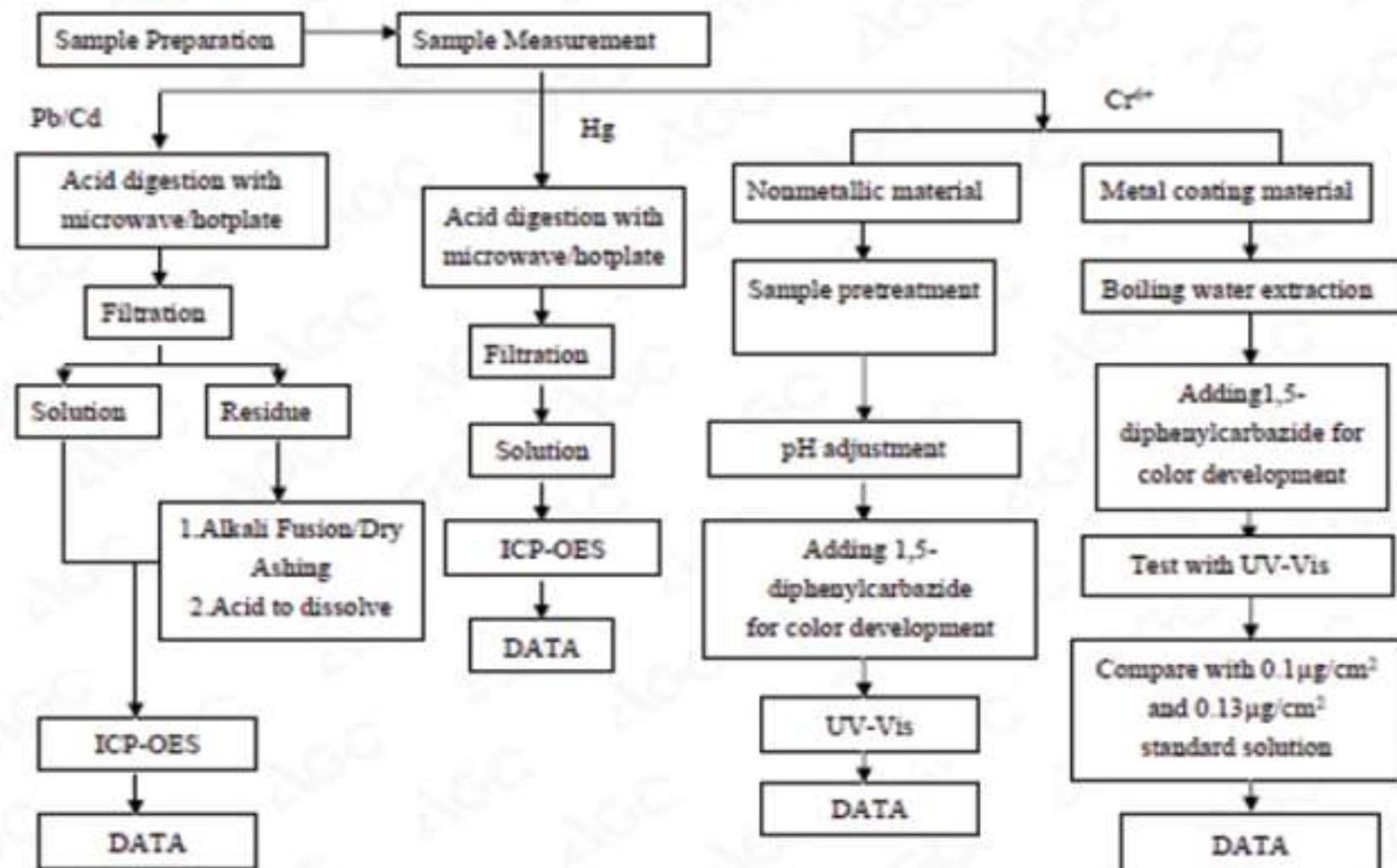
These samples were dissolved totally by pre-conditioning method according to above flow chart (Cr<sup>6+</sup> test method excluded)
