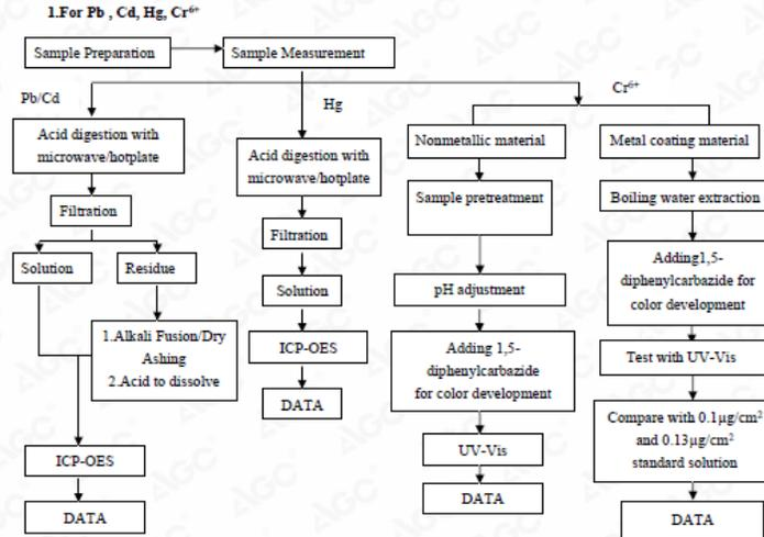
These sample were dissolved totally by pre-conditioning method according to above flow chart (Cr<sup>6+</sup> test method excluded)
